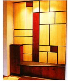
Cubist junkoire. Behind every maple panel in this wall niche is either a door or a drawer activated by a touch latch. The hidden boxes are maple faced with an ebonized edgeband; the accent material is bee's-wing figured andiroba. Design, construction, and photo by Jon Frost of St. Paul, Minn.
